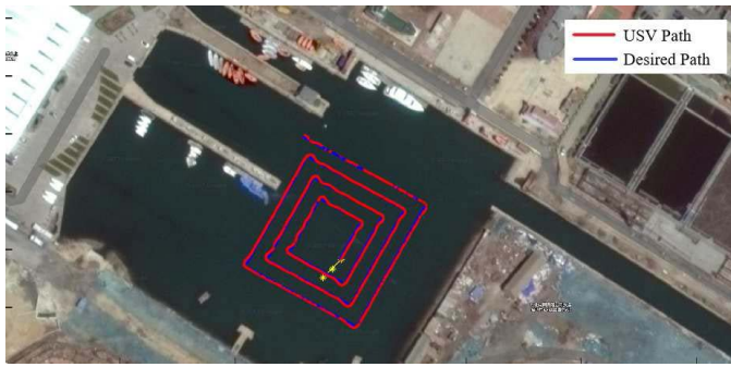
Fig. 4. Tracking performance of the CSICET-DH01 USV in the experiment.
