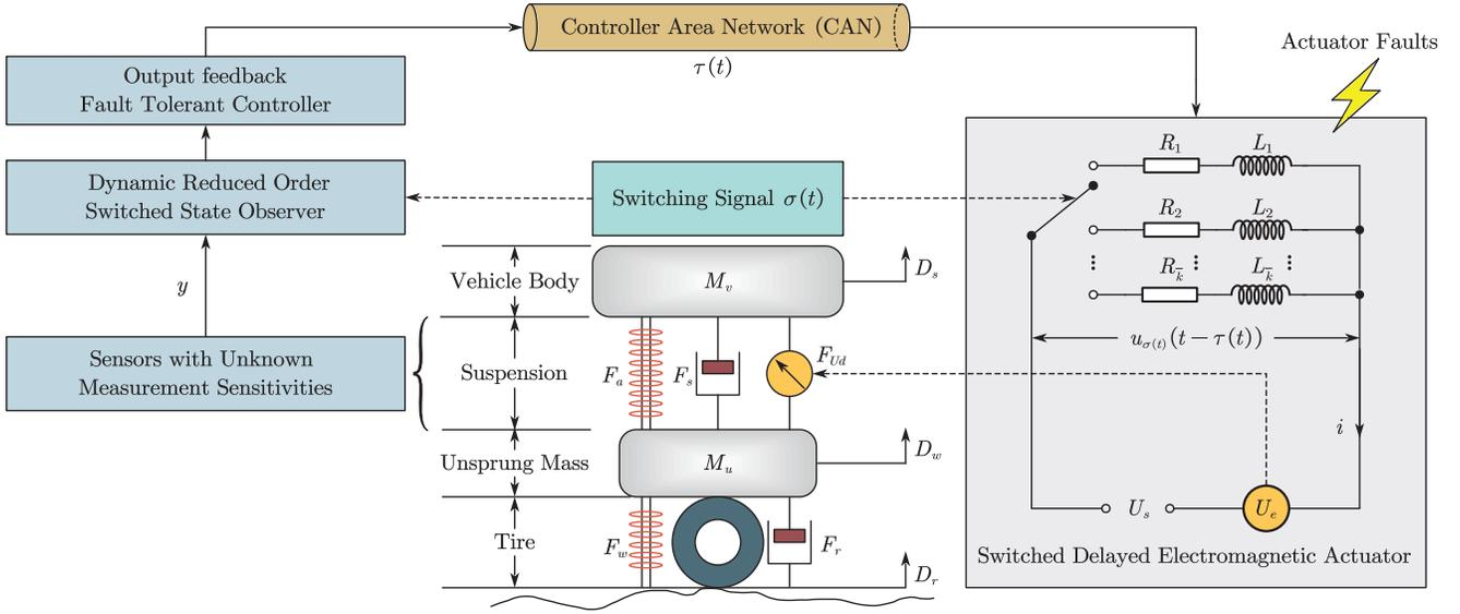
Fig. 1: The framework of switched vehicle active suspension delayed systems over the CAN.
