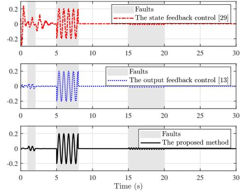
Fig. 12: The designed control input  $u_k$  under actuator faults of the different strategies.
