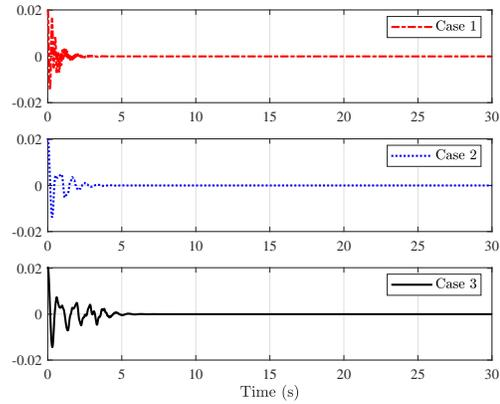
Fig. 4: The suspension space  $x_1$  of Cases 1-3.
