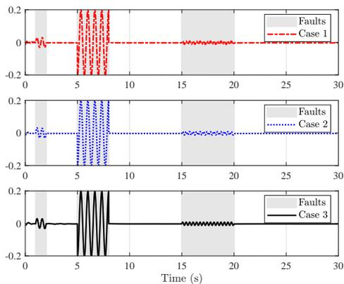
Fig. 7: The designed control input  $u_k$  under actuator faults of Cases 1-3.
