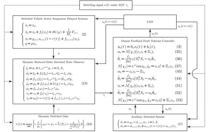
Fig. 3: The block diagram of the proposed control scheme.
